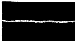
Oscillogram showing noiseless performance of Bradleyunit Resistors.
